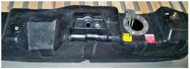
(Fig. 4) This photo shows the venting accommodation for the tank. Use the stock tank's fill and vent hose to attach to the king fill and vent nipples shown in the center. No additional hose is needed. This is how the tank comes out of the box.
