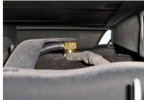
(Fig. 5) Install rubber bushings (pn 99 0000 0103) on both straps with the channel side toward the strap.
