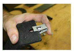
(Fig. 3) If vehicle has threaded clips, remove them from the OEM straps and place them on the TITAN straps.
