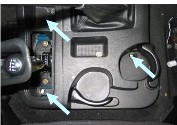
Remove the inner shifter boot with an 8mm socket.
