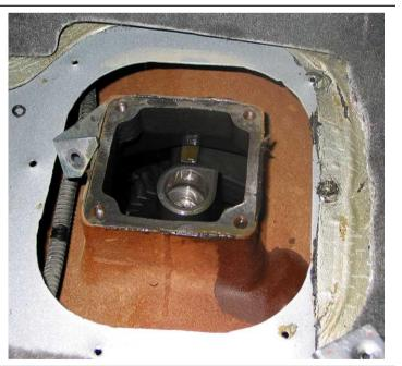
Using a number T-25 Torx bit, disassemble the shift tower.
