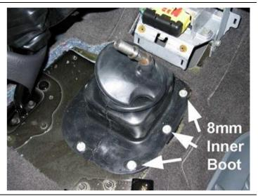
Remove the shift tower from the transmission.
