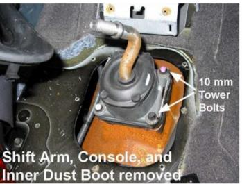
Clean up any residual silicone gasket material from the top of isolator and the transmission case.
