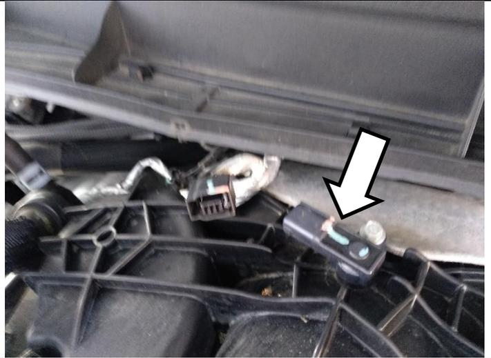
Plug the supplied wiring harness MAP sensor connector inline.
