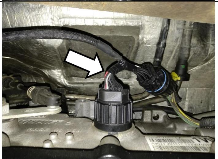
Install supplied zip-ties to support the wiring harness between the engine bay and transmission.
