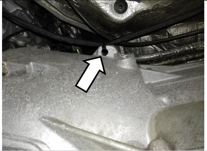
Locate the factory MAP sensor on the top of the intake manifold. Unplug the sensor connector.
