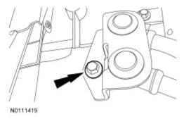
35. Remove the lowers transmission fluid filler tube bolt and position and transmission fluid filler tube aside. Remove and discard the transmission fluid filler tube Oring.
