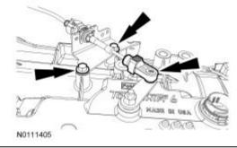
30. Install the transmission vehicle harness connector and lock the transmission vehicle harness connector by rotating the outer shell clockwise.
