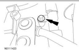
Inspect the transmission fluid cooler tube O-rings for damage and install new O-rings as necessary. Lubricate the O-rings with clean transmission fluid.
