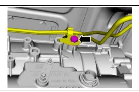
28. Position the wiring harness and install the retainer in the transmission case.
