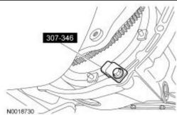
Position the transmission on the dowel pins on the back of the engine. Install the 11 bolts. Tighten to 48 Nm (35 ft-lb).
