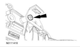
Position the transfer case linkage and install the bolt. Tighten to 115 Nm (85 ft-lb).
