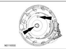
3. Install the Torque Converter
