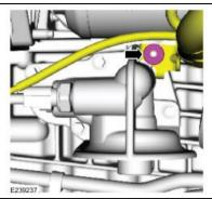
40. Connect the oil temperature sensor and oil pressure switch electrical connectors.
