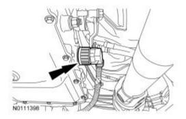
17. Disconnect the selector lever cable end from the manual control lever, remove the 2 bolts and position selector lever cable and bracket aside.
