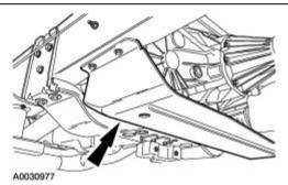
25. Install LH engine support insulator nuts. Tighten to 200 Nm (148 ft-lb).
