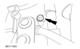
36. Remove the 11 bolts and remove the transmission from the engine dowel pins.
