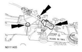
18. For **2017-2019** trucks remove the bolt for the fuel line bracket and position aside.
