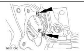
7. Install a new transmission fluid filler tube O-ring. Lubricate it with clean transmission fluid.
