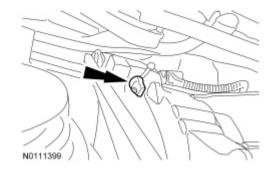
20. Remove the 4 RH engine support insulator nuts.
