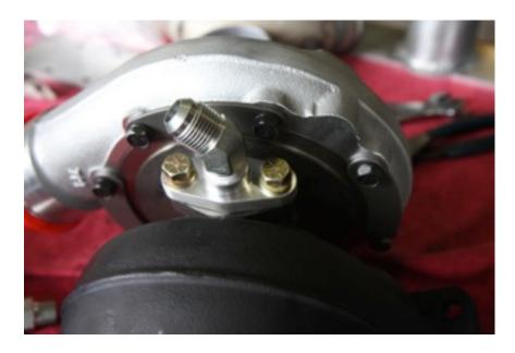
8. Install turbo to collector. You can now install the oil supply and drain lines. The fittings and flanges will need to be installed in the turbo and the drain flange and aligned properly to line up.
