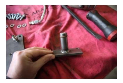
3. Once all old turbo system components are removed. Install the pedestal plate in the valley of the engine using the supplied 8x25mm bolts (4).
