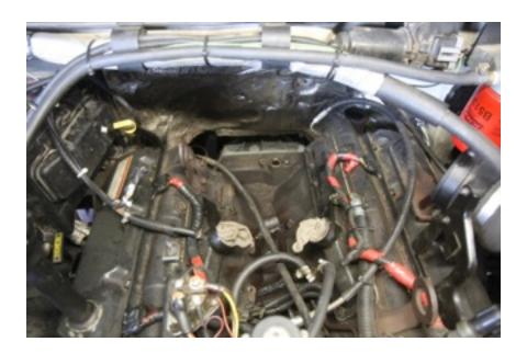
2. If installing turbo on Superduty truck remove the soft plug from the valley and install the oil drain fitting using two supplied 8x25mm bolts. If installing in a superduty than the soft plug in the valley needs to be removed. This can be done by drilling a small hole and then installing a screw into the hole and grabbing with pliers to ensure it doesn't fall into the motor. It may be necessary to tap gently to break it loose.
