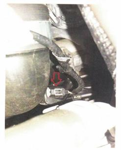
7. Reroute the charge air temperature sensor connector under the upper radiator hose and plug it into the SOTF cable adjacent to the battery (as depicted below). Route the SOTF cable between the battery and fender. Pull any excess slack in the SOTF cable from the engine compartment into the cab.
