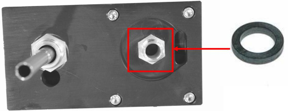
**Note: O-Ring must be put back on suction side of pump. Failure to do so can result in priming issues, cavitation, or pressure loses.**
