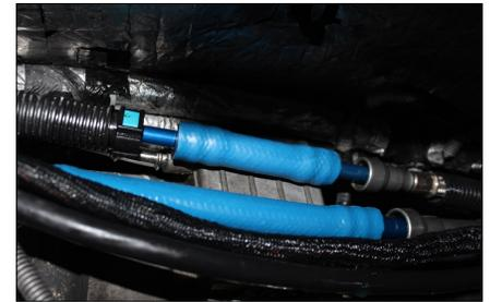
**Note: Secure all fuel lines with cable ties. Cable ties are an economical way to prevent the possibility of problems occurring!**
