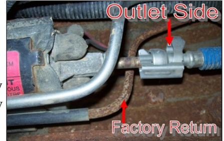
H. Route the fuel line from the “E” port of the FASS to the factory lift pump’s quick disconnect and cut to length. Insert the PLB-12516 into FASS fuel line using oil. Slide the PLB-12516 into the factory quick disconnect until you hear a click. Lock down factory retainer clip.
