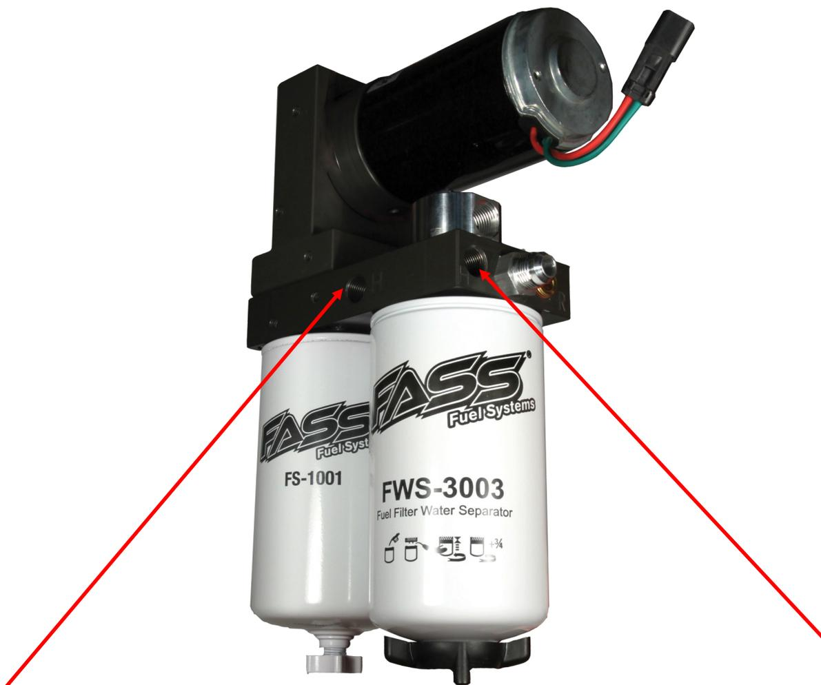
**Note: The Red Plastic Plugs located in the “H” ports can stay in place fuel will not flow through these ports. Coolant can be plumbed into these ports to heat the fuel in the Winter months.**
