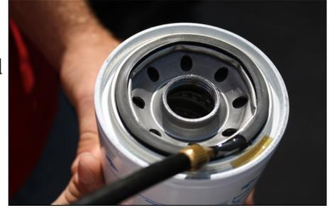
**Fuel Filter –Install FWS-3003 on side of pump with draw tube in the middle of the filter nipple.**
