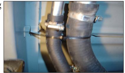
**Helpful Hint: If more space is required to access the top of the fuel tank, loosen the strap nuts to the end of the stud. This will gain you about 3" more working room.**
