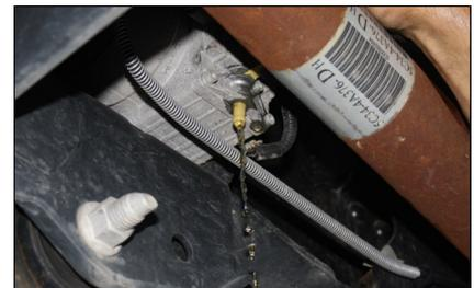
H. Using quick disconnect tools, remove the fuel lines from the front of the factory fuel pump. Remove the fuel lines attached to the rear of the factory fuel pump by pressing in on the tabs.
