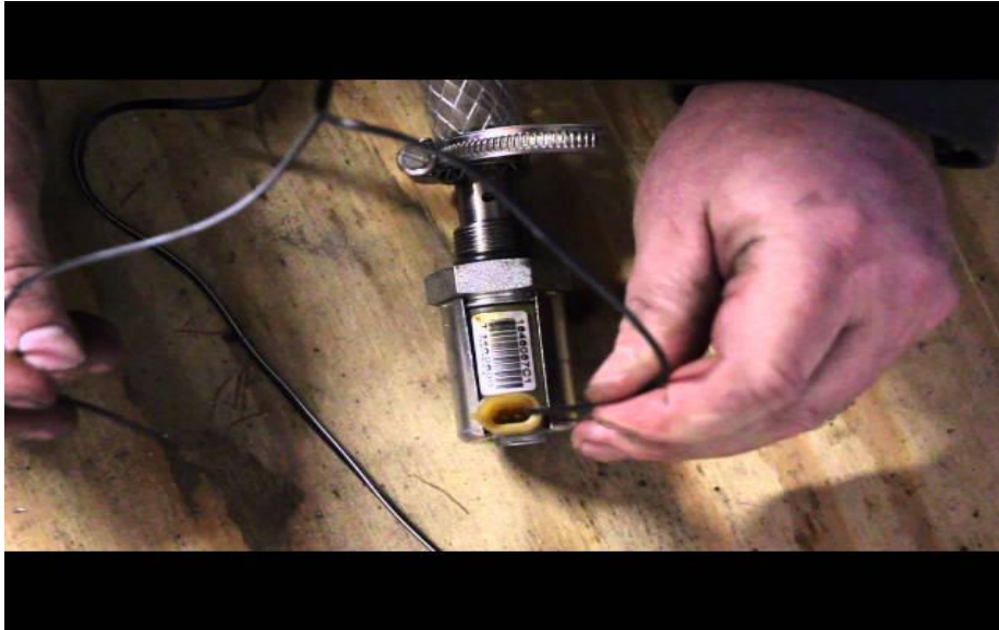
Bench testing the IPR solenoid and valve function
