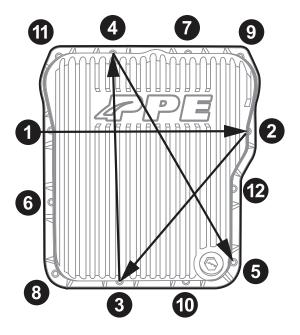
Fill with recommended fluid. Check for leaks.
