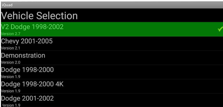
Other vehicle selections are for legacy modules, tunes, and board modifications. You must have the matching software and hardware in order to run different vehicle profiles. "V2 Quadzilla Only" is for internal company use and testing only.
