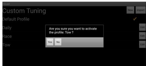
The tune profile currently running on your Adrenaline will be identified by the check mark at all times. To edit a tune profile touch the edit button to the right of the screen. To delete a tune profile touch the trash can in the lower left hand corner of the screen, then touch the red minus sign beside the tune profile you wish to delete. Follow this by touching the red delete button and follow any on screen prompts.
